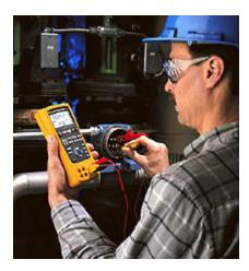
Take along the new Fluke 725 Multifunction Process Calibrator, and you're equipped to test and calibrate almost any process parameter. Measure and source mA, volts, temperature (RTDs and thermocouples), frequency, ohms, and pressure, using optional pressure modules.
