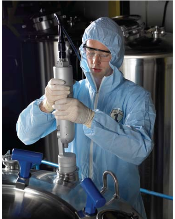
Pharmaceutical tank inspection through 76 mm (3.0 in) \emptyset nozzle
