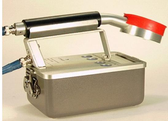
The 4 soft-key buttons on the front panel operate the instrument. The two on the right are user defined. One user may want to use them for light and beeper while another may want to use them for range hold and reset. The soft-keys also help to simplify the operation of the instrument. There is only one level of display; you are never lost in a maze of menus.
