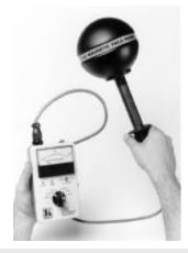
Isotropic Response True RMS Detection 100dB Dynamic Range
